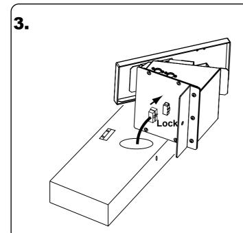
Plug in the key scan cable from the Pedal Keyboard to the Expression Pedal.
