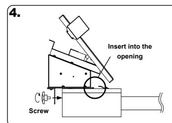
Mount the Expression Pedal on the Pedal Keyboard using the Screw (knob bolt).
