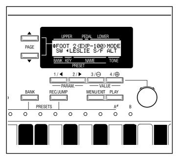
The Foot Switch is used to operate and control the organ by your foot instead of pressing various switches by hand while playing. The initial factory assignment is "LESLIE FAST".
